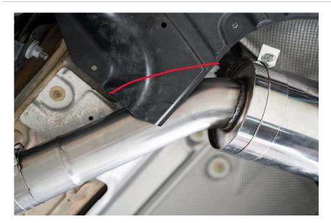
The undertray also requires trimming to clear the exhaust. The red line indicates the amount to be removed.
