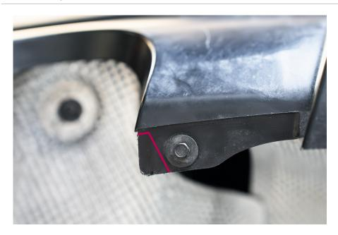
The rear bumper requires trimming for the L/H outlet. The red line on the 1st image indicates the position.
